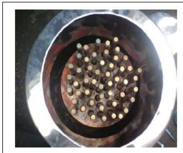
Figure 2: Fabricated PCM's Storage Tank
